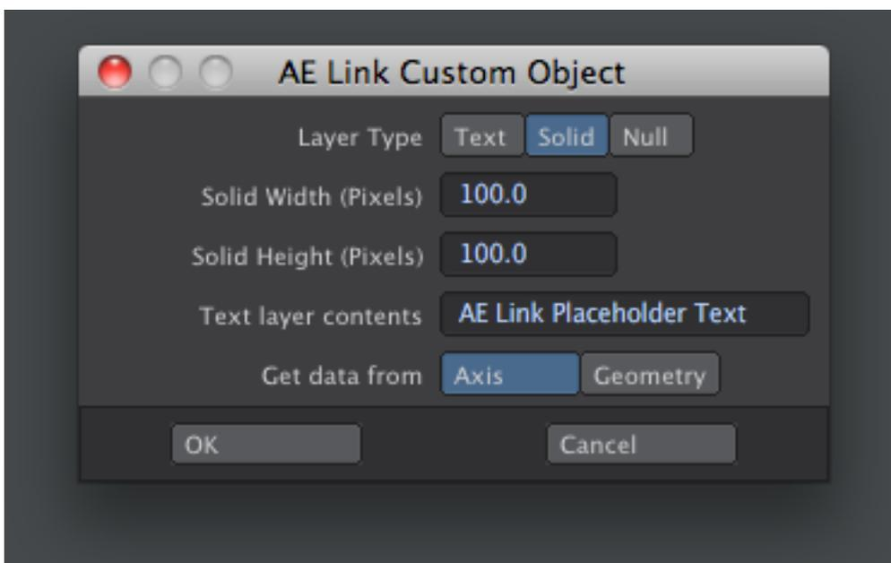
“Layer Type” allows to set how After Effects will use this object. It defaults to “Solid” and will create a solid using the “Solid Width” and “Solid Height” values specified in this panel.
